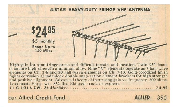
From the same 1969 Allied Radio catalog, the VHF antenna pictured above is a variant of a log periodic antenna. At channels 2 to 6, the elements serve as a standard log periodic. At channel 7 to 13 the antenna functions as a 3/2 wavelength or third harmonic mode design. The three elements in the front are directors. The elements are swept forward for slightly more gain.
